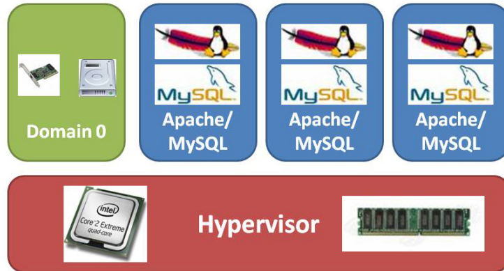
Figure 3.2: VPS Hosting Workload Architecture. A high-level view of the VPS application workload.
