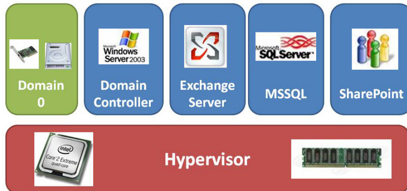
Figure 3.3: Windows Domain Workload Architecture. A high-level view of the windows domain application workload.
